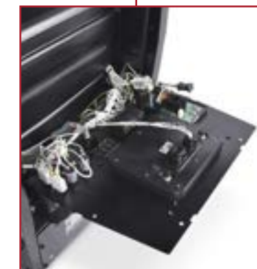
Coated, strain-relief wiring harnesses help connections last longer
